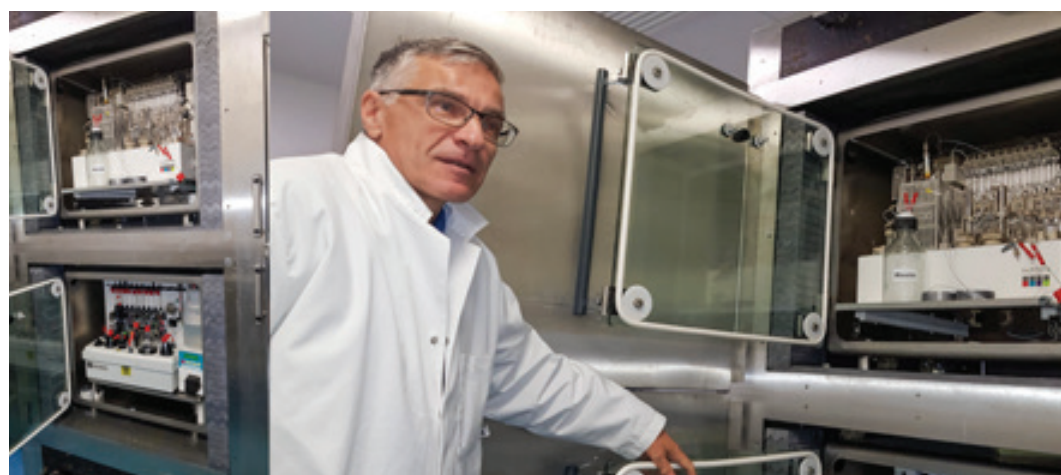
Figure 1 Radioactive hot-cells at the PET Radiopharmaceutical Production Unit at Gartnavel Royal Hospital containing one of the new state-of-the-art Synthra Wolpertinger modules (top left and right) and the refurbished GE Tracerlab (bottom left) with Dr Dmitry Soloviev, Senior PET Chemist. The Synthra Wolpertinger can make any ^{11}\text{C} - or ^{18}\text{F} -labelled metabolite, and the GE Tracerlab is used for research fluorinations. These different modules can be run in quick succession for near simultaneous production of ^{11}\text{C} and ^{18}\text{F} products for research use.
